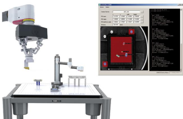
Fig. 1: A hybrid assembly setup consisting of a SCARA kinematic and an attached micromanipulator is shown. The system is mounted on a breadboard which can be equipped to satisfy the needs of laser assembly tasks.
