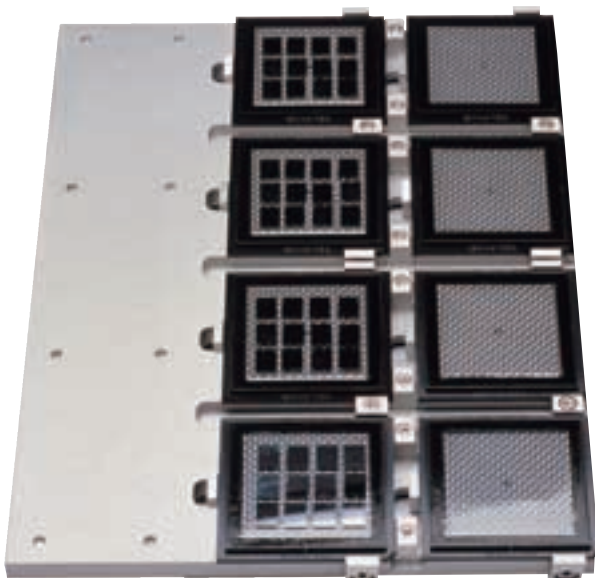
Automated Pick & Place Fixture
