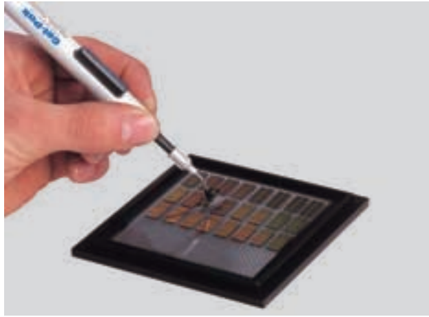
Unloading of Device from VR-44 Tray Using Vacuum Pen
