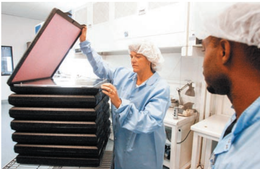
Inspection of a 300mm Large Format VR Plate during the production process.
